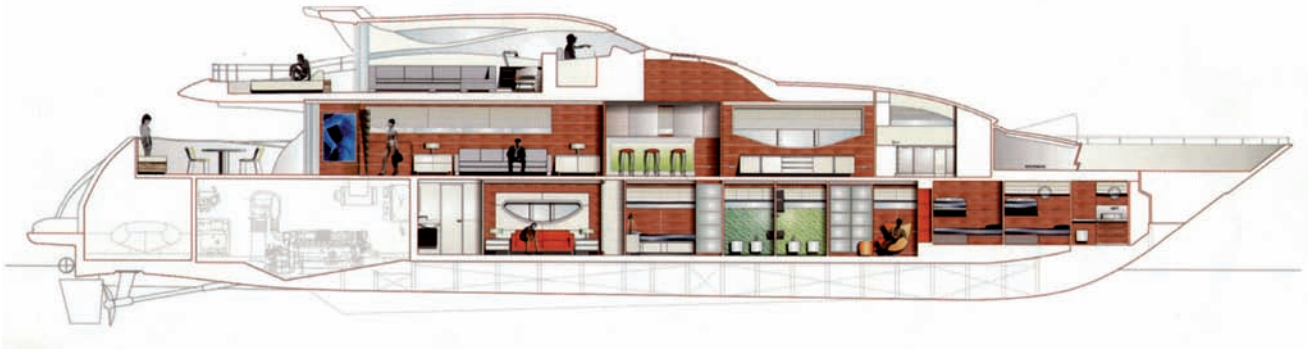
Planet 120. Longitudinal front elevation section. Versilcraft Shipyard. Ñ
